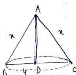
$$\begin{aligned} AD &= \text{altitude} = \sqrt{x^2 - \left(\frac{y}{2}\right)^2} \\ &= \frac{\sqrt{4x^2 - y^2}}{2} \end{aligned}$$
