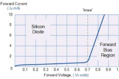
The application of a forward biasing voltage on the junction diode results in the depletion layer becoming very thin and narrow which represents a low impedance path through the junction thereby allowing high currents to flow. The point at which this sudden increase in current takes place is represented on the static I-V characteristics curve above as the "knee" point.
