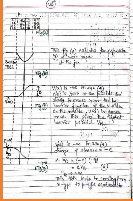
VB 2 barrier fortential. e = change then Energy Ep = eVp This energy En transfer an electron from n-side to the b-side Barrier Energy charge of an electron being negative of the fotential energy EBY an electron obtained Explanation in
