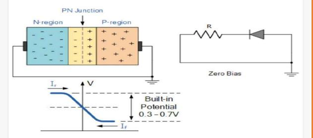
The potential barrier that now exists discourages the diffusion of any more majority carriers across the junction. However, the potential barrier helps minority carriers (few free electrons in the P-region and few holes in the N-region) to drift across the junction.
