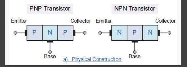
The **Bipolar Transistor** basic construction consists of two PN-junctions producing three connecting terminals with each terminal being given a name to identify it from the other two. These three terminals are known and labelled as the Emitter (E), the Base (B) and the Collector (C) respectively.
