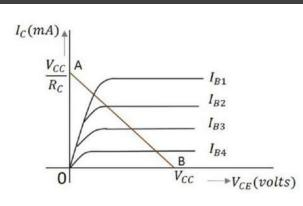
To obtain the load line, the two end points of the straight line are to be determined. Let those two points be A and B.
